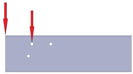
\*\*\*CUT FACTORY FRAME RAILS OFF AT 4 3/8 INCHES FORWARD FROM CENTER OF FACTORY RIVET HOLE REFERENCED IN IMAGE ABOVE\*\*\*
