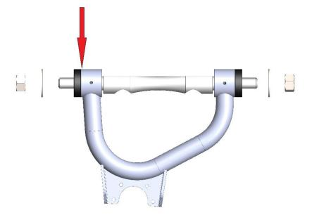
Once the bushing is fully seated, tighten the nyloc nut until the washer bottoms out against the machined shoulder on the cross-shaft. Then tighten 1/4 turn.
