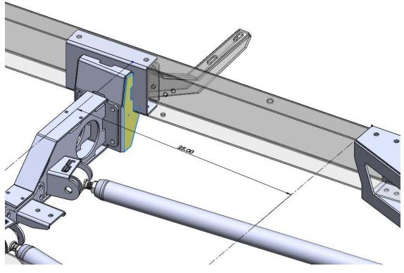
FRONT EDGE OF TRAILING ARM CROSSMEMBER BRACKET (IN YELLOW) WILL SET 25 INCHES FORWARD OF THE NOTCHES FRONT EDGE (SEE PIC BELOW) MARK AND DRILL HOLES, INSTALL USING SUPPLIED GRADE 8 HARDWARE; TORQUE TO 65 FT LBS
