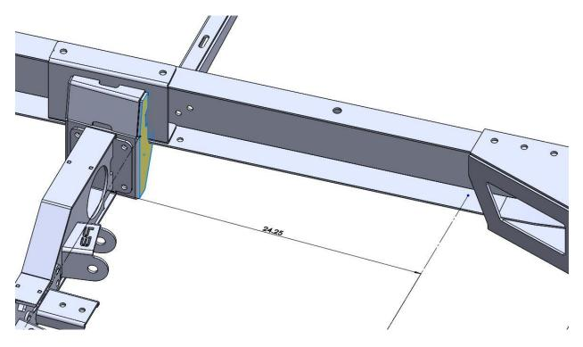
FRONT EDGE OF TRAILING ARM CROSSMEMBER BRACKET (IN YELLOW) WILL SET 24.25 INCHES FORWARD OF THE NOTCHES FRONT EDGE (SEE PIC BELOW) MARK AND DRILL HOLES, INSTALL USING SUPPLIED GRADE 8 HARDWARE; TORQUE TO 65 FT LBS
