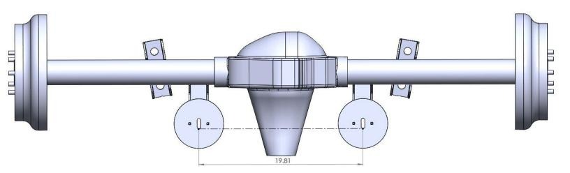
SET THE LOWER AIRBAG BRACKETS' MOUNTING FACE PERPENDICULAR TO THE PINION
