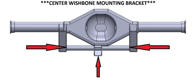
WISHBONE MOUNTING BRACKET WILL ATTACH TO SPREADER TUBE AND BOTTOM OF AXLE HOUSING (TRIMMING MAY BE NECESSARY FOR PRECISE FITMENT)
