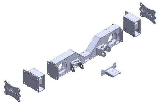
\*\*\*NOTCH IN BRACKET INDICATES TOP AND FRONT MOUNTING ORIENTATION\*\*\*
