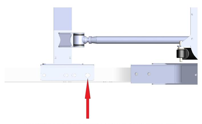
73-87 INBOARD 4 LINK CROSSMEMBER FRAME C-CHANNEL WILL ALIGN WITH FACTORY BED MOUNTING HOLE REFERENCED MY ARROW
