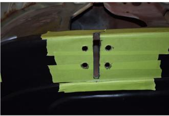
Mount the pocket and gas strut braces. Don't tighten the hardware yet. Note the orientation of the strut brackets.
