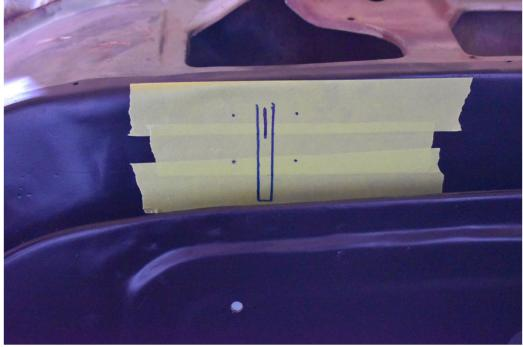
Using a punch, mark the holes on the firewall and bottom of the hood hinge slot.
