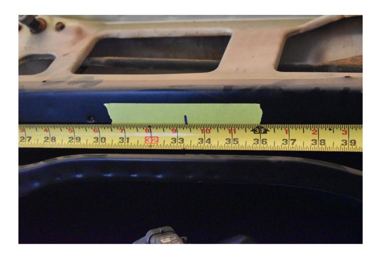
Once the center point is marked, measure 23" to the driver side and passenger side. Apply a few pieces of tape to the firewall before marking these points.
