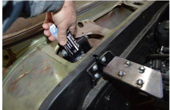
Install the hood hinge plates to the hood hinge. Grind the top and bottom edges (shown with a blue mark) to prep them for welding.
