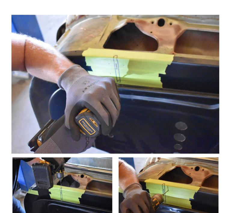
After drilling pilot holes, use the 5/16" bit and drill out the bottom and top of the hood hinge slot. Drill the 4 bolt holes as well.
