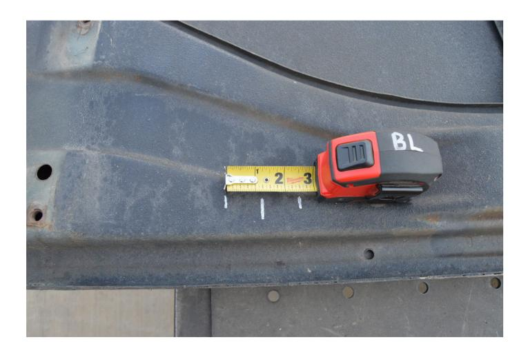
Mark an additional  $\frac{1}{2}$ " on each side. Using a square, extend the lines toward the front of the hood. This will be the area to prep.Be sure to clean/prep the surface down to bare metal, as shown in the photo.
