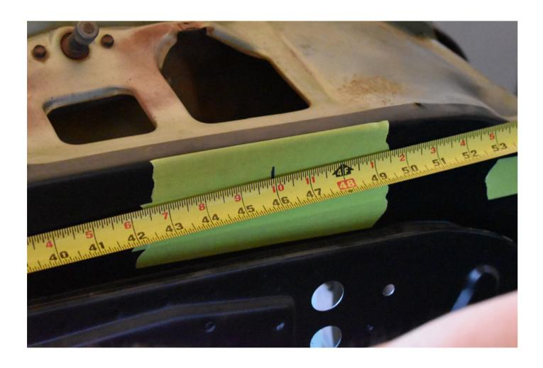
We're now ready to use the hood hinge pocket templates created earlier. Starting with the passenger side, flip the template over and align the center line with the measurement from the previous step.
