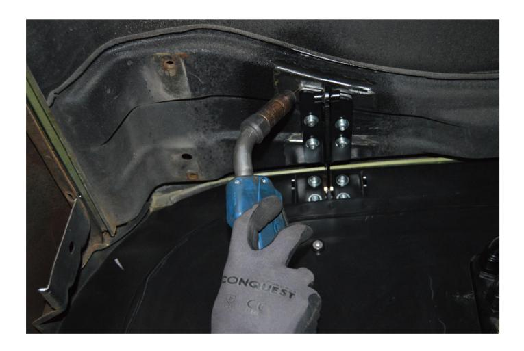
With the plates tacked to the hood, remove the hardware holding the plate to the hinge arms and remove the hood from the vehicle.
