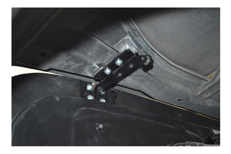
This next step can be completed a few different ways. The preferred method is to tack the plates onto the hood with the hood in place on the vehicle. Alternatively, the hood hinge plate location can be traced with a Sharpie or other permanent marker, then remove the hood and tack/weld the plates in place.
