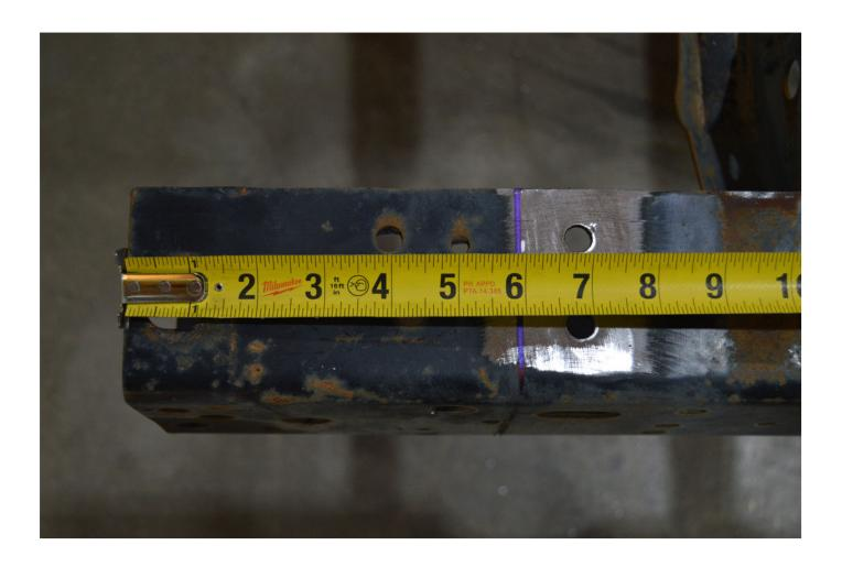
The template can be used to mark or score the cut line, if need be.
