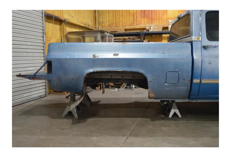
With the bed installed and aligned, mark the hole location with a Sharpie.
