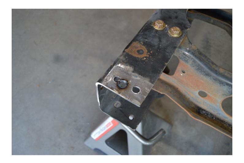
If you don't want to install and remove the bed again, the rear frame rail sections can be used to mark the bed hole location. Flip the trimmed piece upside down and place it on top of the opposite frame rail. Align the rear and inside edge, then mark the bed mounting hole location.
