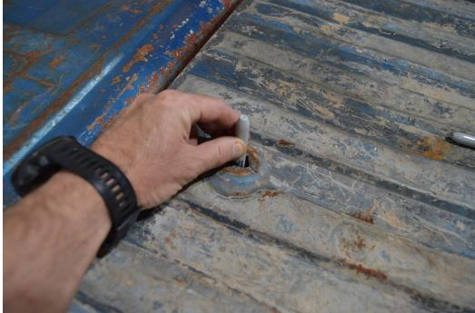
Remove the bed and drill the hole with a ½" drill bit.
