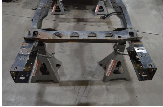
Use a 7/16" drill bit to enlarge the existing factory holes or drill the new holes.
