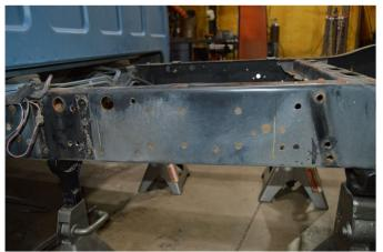
With the bracket removed, prep the frame around the cut lines using an angle grinder and a flap disc. This section of the frame will get welded in a later step.
