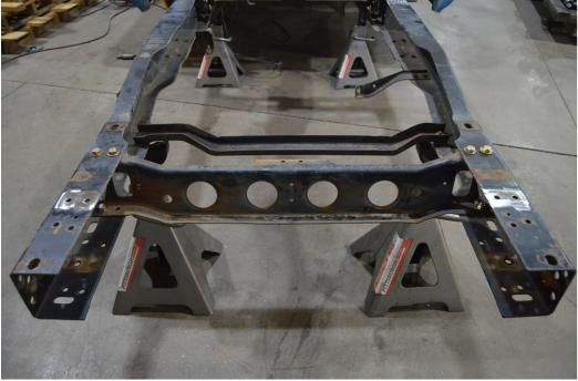
Lay the template sideways on top of the rear frame rail and align the back edge as shown. Mark the frame rail with a sharpie. Clamp the template to the side of the frame or use the square to transfer the mark to the side of the frame.
