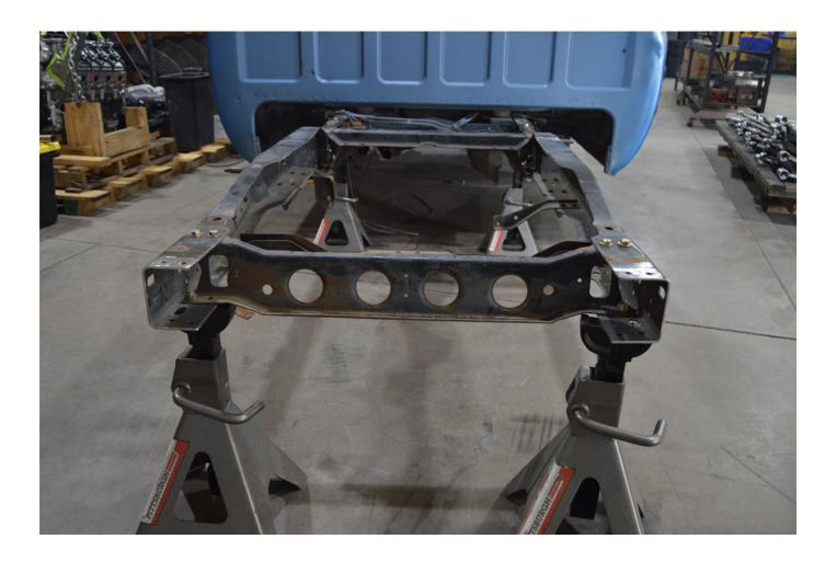
The last step is to mark and drill the rear most bed mounting hole locations.
