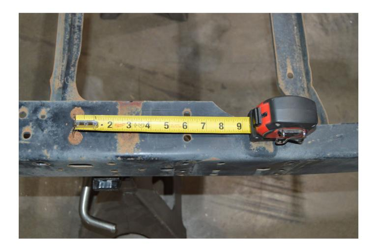
Remove the factory rear frame crossmember and bolt it into the new location 6" forward.
