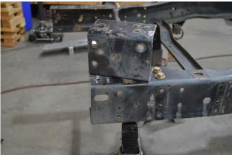
Here's the frame with the rear section trimmed and removed.
