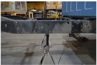
Using a 7/16" drill bit, drill out the 4 factory holes for the front leaf spring hanger. The template will bolt into these holes.
