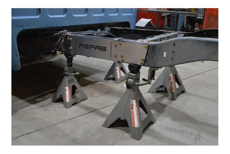
With the bracket installed, it's time to mark the cut lines. This can be done by using a pen, small screwdriver, or tool to score the frame. An angle grinder with a cut off wheel can also be used.
