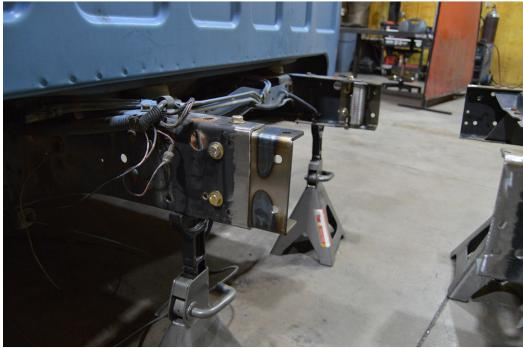
Slide the rear section on to the c-channel pieces and bolt it in place.
