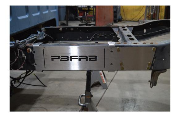
Now that the template is bolted in place, drill out the remaining holes. Be sure not to skip the holes on the top and bottom of the frame.
