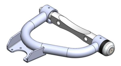
INSTALL OTHER BUSHING IN CONTROL ARM. IT MAY BE NECESSARY TO PRESS THE BUSHING IN PLACE.
