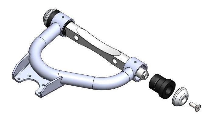
INSTALL ONE BUSHING IN THE CONTROL ARM. MAKE SURE THAT THE BUSHING IS SEATED FLUSH AGAINST THE MACHINED SURFACE OF THE TUBE. (IT MAY BE NECESSARY TO PRESS THE BUSHING IN PLACE)
