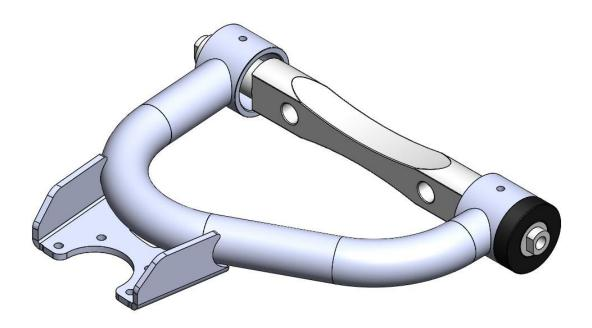
INSTALL BUSHING RETAINER AND 3/8 ALLEN HEAD BOLT; DO NOT YET TIGHTEN.
